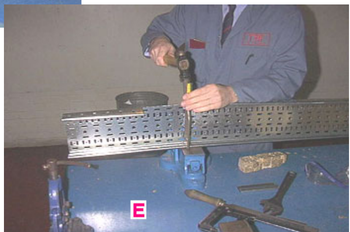
Figure 87: Construct a flat Bend 90° (E)
