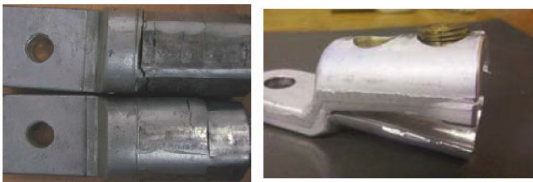
Figure 192: “Problems” with Crimping...
