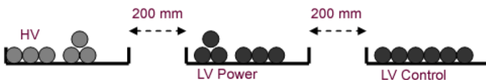
Figure 72: Horizontal distances between cable trays
