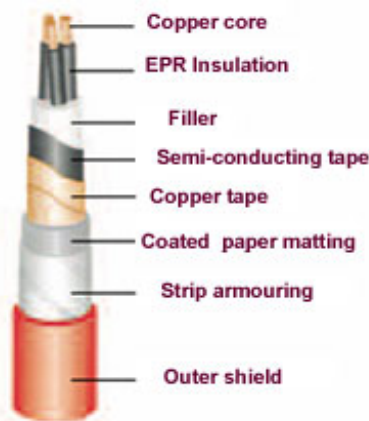
Figure 67: Three-pole armoured cable with a non-radial field, 6kV
