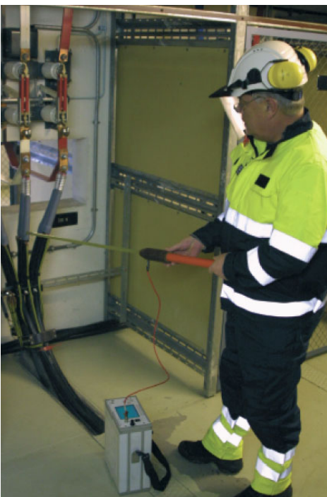
Figure 151: On-line testing of HV cable heads
