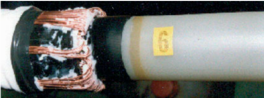
Figure 150: Fault on single-pole 24kV cable
